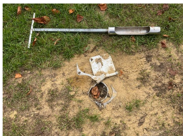
Figure 42: The vehicles which accessed the field have caused considerable damage to the goalpost sockets and severely compacted the impacted underlying soils.
